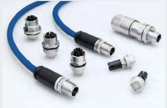
As 8-pole, X-coded compact connectors in Cat.6<sub>A</sub>, the M12 from Telegärtner can transmit data rates of up to 10 Gbit/s in accordance with IEC 61076-2-109:2014. Even in harsh environments, the high bandwidth is ensured by separating the four pairs with a cross shield (X-coding). Remote powering of end devices is also possible.
